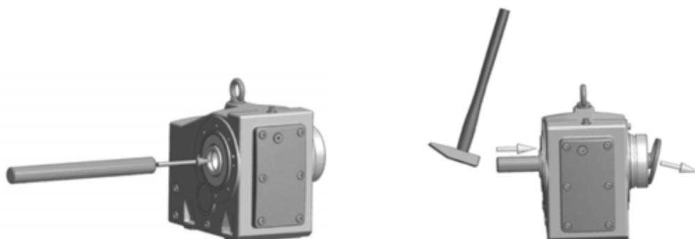
Fig. 6: Removing the factory-fitted closing cap
