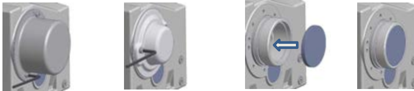
Fig. 13: Fitting the covers, Option SH, Option H, and Option H66
