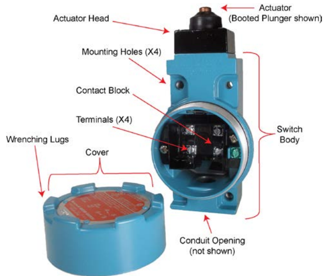
Figure 1. MICRO SWITCH™ LSX Terminology
